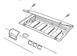
Figure 2-7. Accessing the Memory Slot
